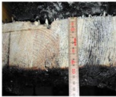
Figure 58: Remaining wood cross section in the joint area of melted boards
