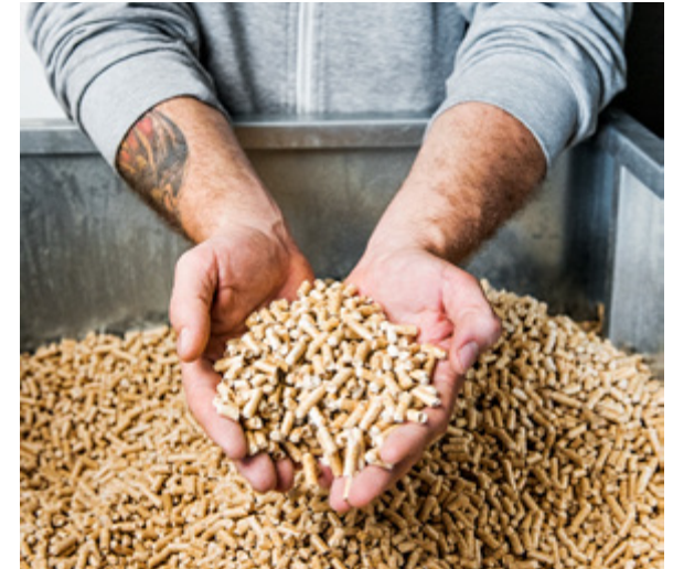
Pellets are made from sawmill by-products and provide a cost-effective and renewable biomass for energy.
