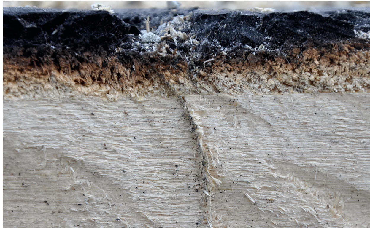
Cross-section surface of a char layer of an 3 1/8" (80 mm)-thick CLT element, originally clad with fire protection plasterboard, after a large-scale fire test: It is easy to identify the different layers on this cross section: the charred area (black area), followed by the pyrolysis area (brown area) — caused by the spreading fire or pyrolysis — and the undamaged wood.
