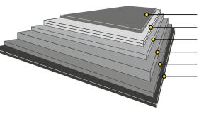
LDPE coating Double pigment coating Bleached chemical pulp Unbleached chemical pulp and CTMP Unbleached chemical pulp LDPE coating
