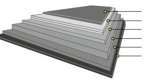
LDPE coating Double pigment coating Bleached chemical pulp Unbleached chemical pulp and CTMP Unbleached chemical pulp LDPE coating
