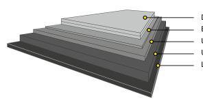
Double pigment coating Bleached chemical pulp Unbleached chemical pulp and CTMP Unbleached chemical pulp LDPE coating
