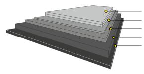
Double pigment coating Bleached chemical pulp Unbleached chemical pulp and CTMP Unbleached chemical pulp LDPE coating
