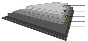
Double pigment coating Bleached chemical pulp Unbleached chemical pulp and CTMP Unbleached chemical pulp LDPE from renewable raw materials
