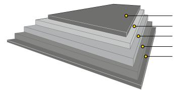
Dispersion barrier Top layer (sulphate pulp) Middle layer (sulphate pulp + CTMP) Back layer (sulphate pulp) Dispersion barrier
