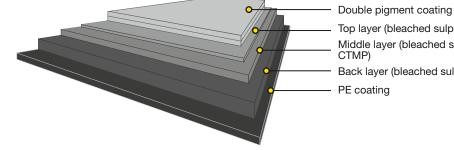
Top layer (bleached sulphate pulp) Middle layer (bleached sulphate pulp + CTMP) Back layer (bleached sulphate pulp) PE coating
