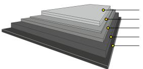
Double pigment coating Chemical pulp Chemical pulp + CTMP Chemical pulp Surface sizing
