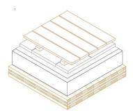
26 mmdecking boards44 mmwooden battens12 mmlevelling pads, sylomer40 mmpaving slabs and macadam2.5 mmEPDM roofing membrane200 mmEPS insulation140 mmCLT by Stora Enso
