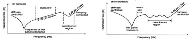
The figure shows the different behaviour of isotropic and orthotropic materials. [4]
