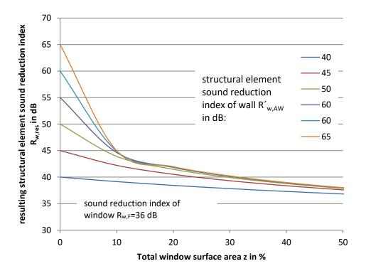
The diagram shows the  $R'_{res,w}$  depending on the window surface area when installing a window with  $R_{w,F} = 36 \text{ dB}$ .
