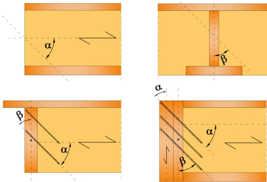
Figure 48: Screw angle  $\alpha$  angle between screw axis and the grain direction and  $\beta$  between the screw axis and the plane parallel to the flat face of LVL.
