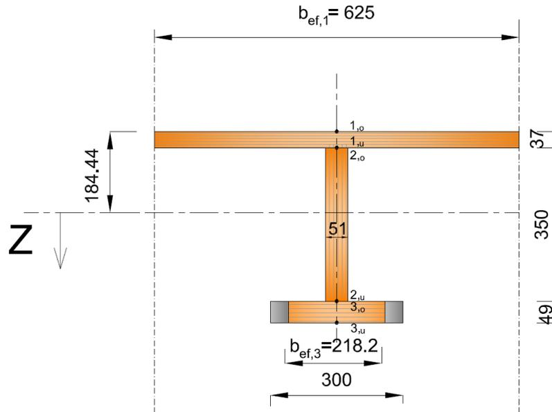
Figure 63: The calculation points of bending stress ( $t = 0$ )
