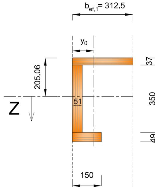
Figure 76: U section in SLS ( $t=0$ )
