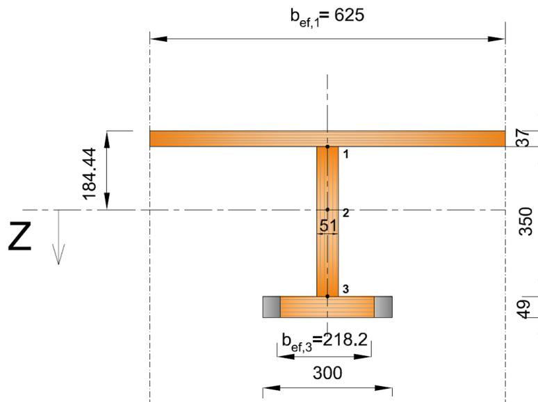
Figure 65. The shear stresses should be calculated in three points
