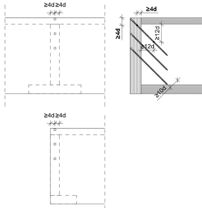
Figure 52: Minimum spacing, end and edge distances. The edge distance to the end of support beam should not be less than  $5d$ .
