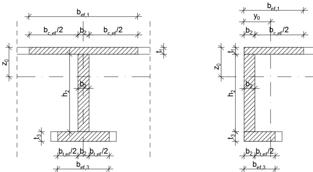
Figure 19: Parts of the effective cross-section and designations used in middle and edge ribs (Slab in compression).
