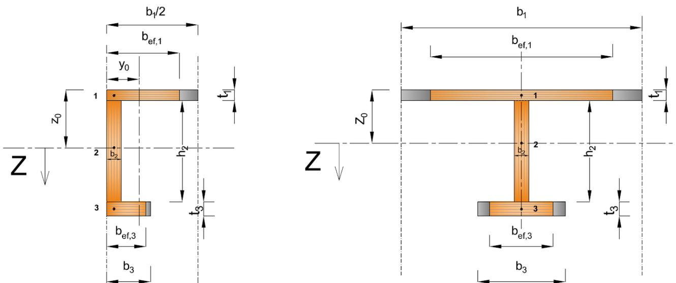
Figure 27: Calculation points of bending stress for rib panel
