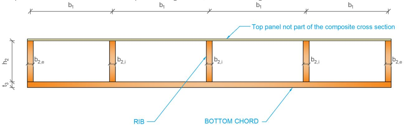
Figure 5: LVL Rib panel- Closed type.
