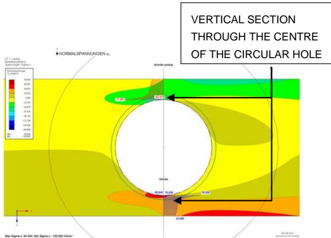
Figure 16: Longitudinal stresses at the contour of the hole and the edge of the beams
