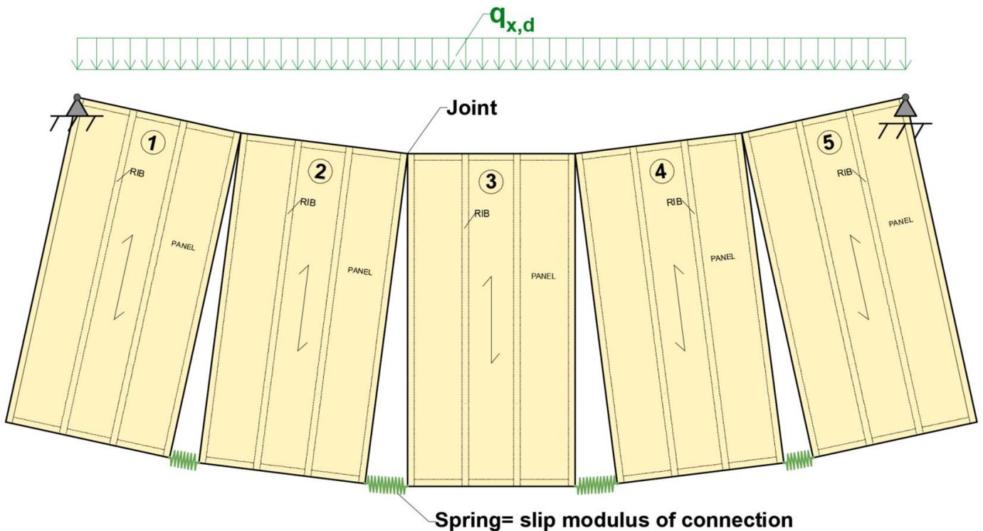
Figure 40: Diaphragm behaviour in longitudinal direction with springs in longitudinal joints at the end of the panels.
