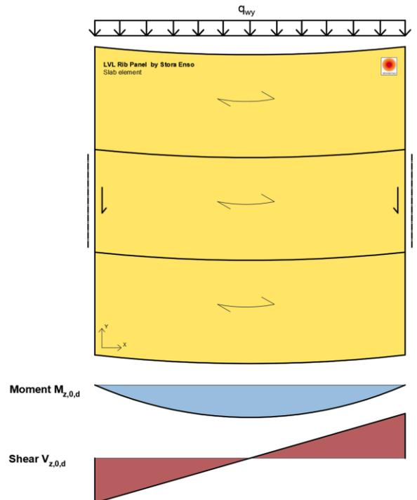
Figure 37: Failure mechanisms of diaphragms
