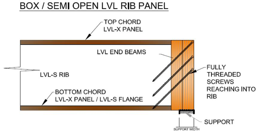
Figure 49 : Example with end beam support
