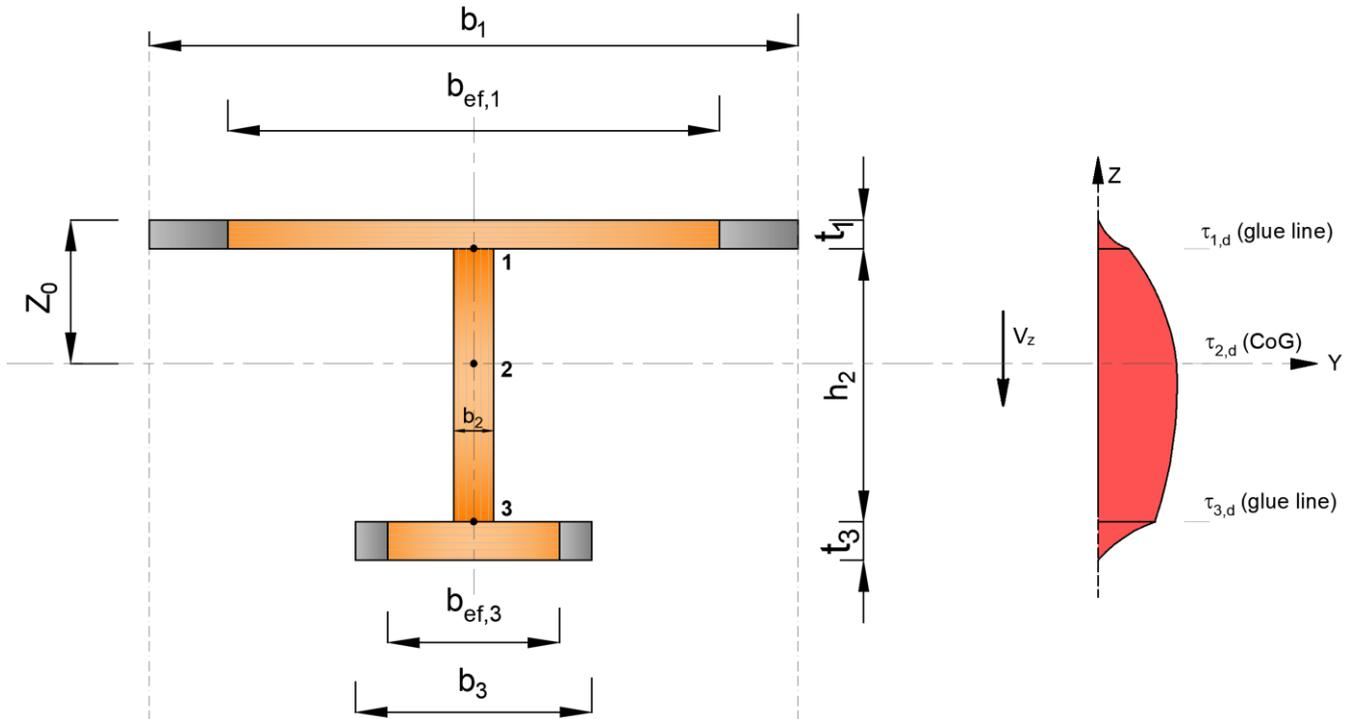
Figure 31: Shear stress distribution
