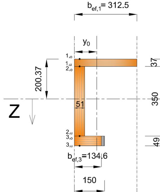
Figure 69: The calculation points of bending stress ( $t=0$ )
