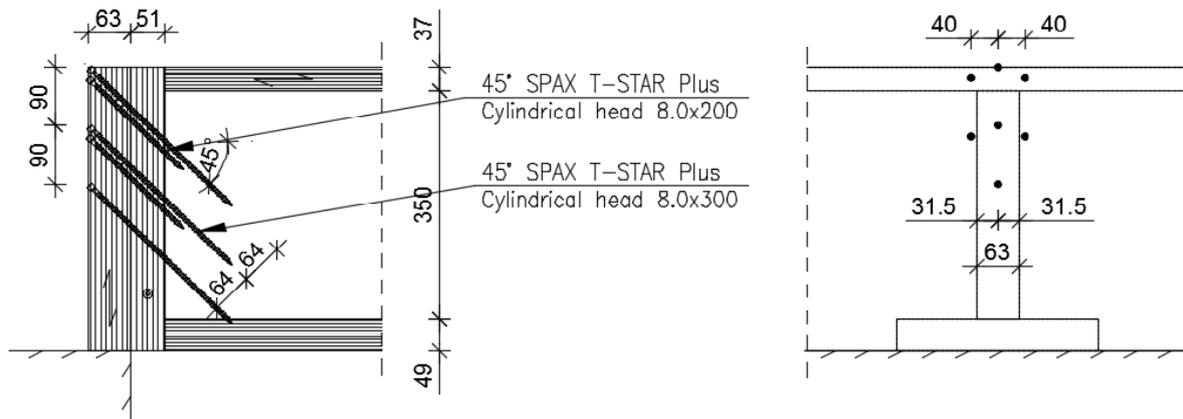
Figure 78: Illustration of an I section end beam support.
