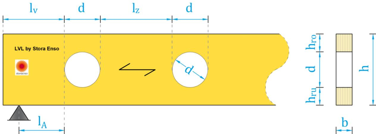
Figure 11: Definitions of geometric dimensions related to circular holes
