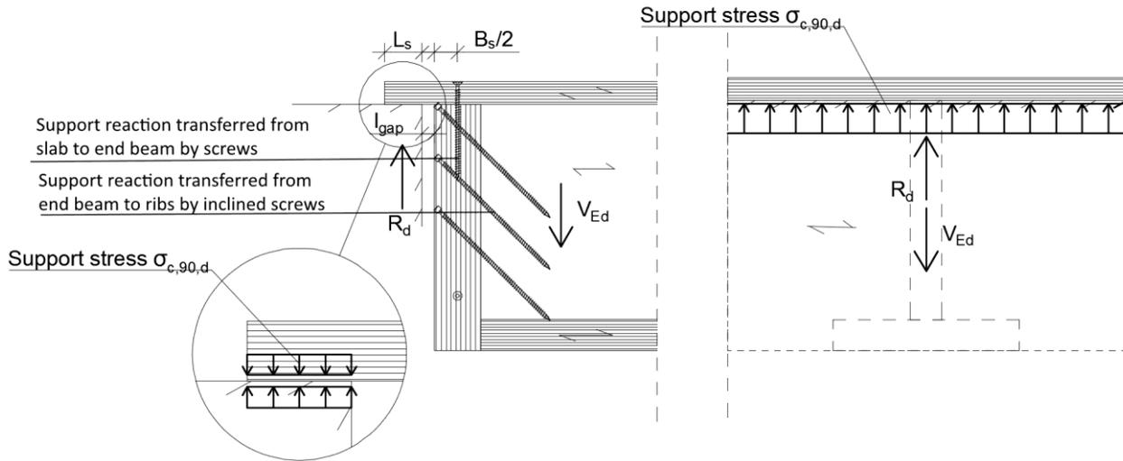
Figure 55: Suspension support. Support reaction is transferred to shear force in ribs through end beam. ( $V_{Ed} = R_d$ )
