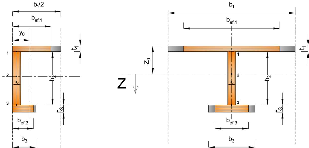
Figure 30: Calculation points of shear stress.
