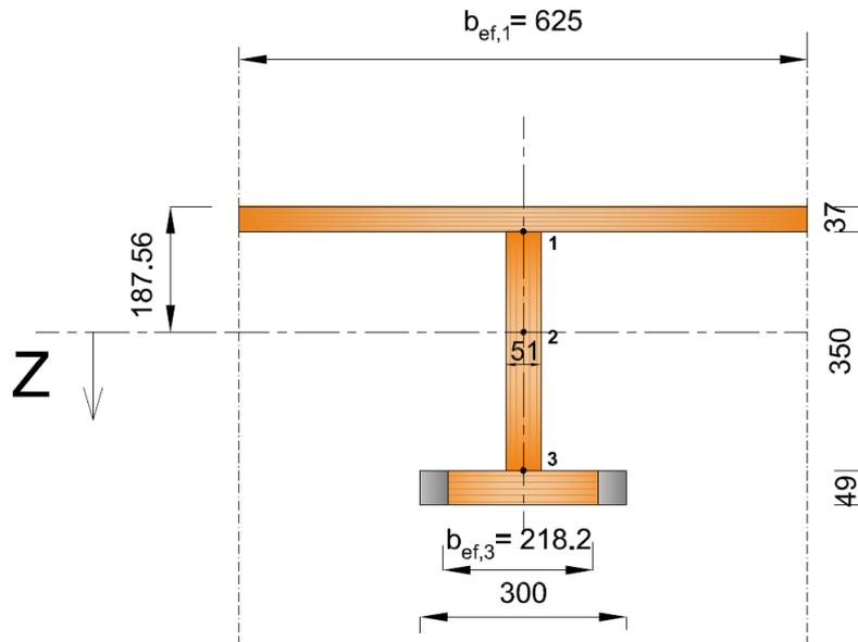
Figure 66: The calculation points of shear stress ( $t = \infty$ )
