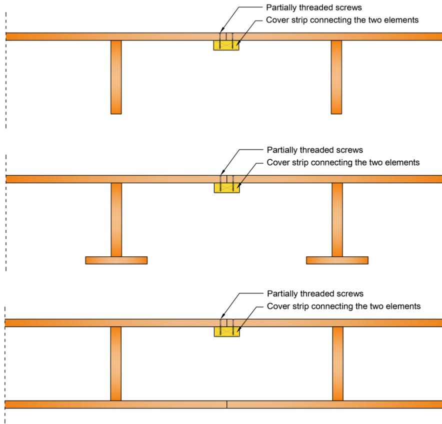
Figure 34: Assembly of adjacent LVL Rib Panels by means of cover strip connection screwed at the LVL plates with edge ribs.
