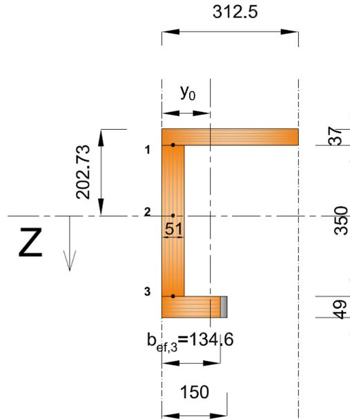
Figure 72: The calculation points of shear stress. ( $t = 0$ )
