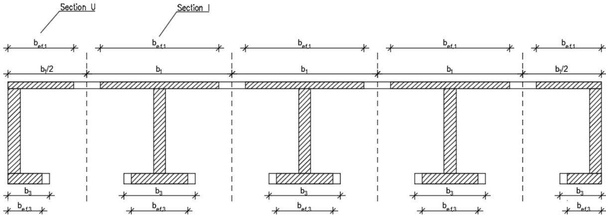
Figure 18: Sections I and U of rib panel (effective areas in bending hatched).
