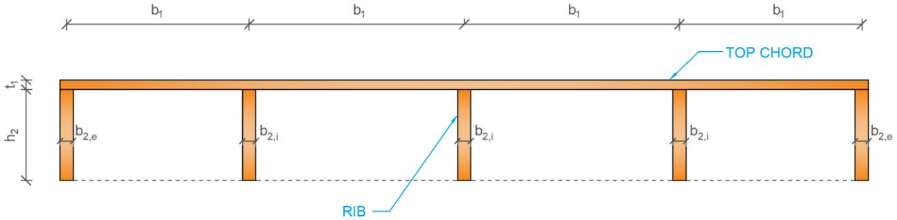
Figure 2: LVL Rib panel- Open type.
