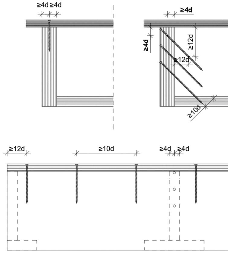
Figure 57: Minimum spacing, end and edge distances.
