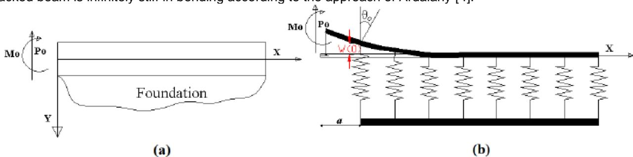
Figure 13 : Model of beam on elastic foundation: (a) beam on elastic foundation, (b) schematization of a beam on springs as elastic foundation, [7].
