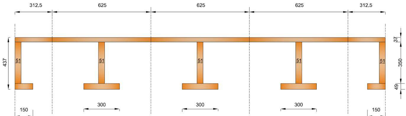
Figure 59: Cross-section of design example panel.
