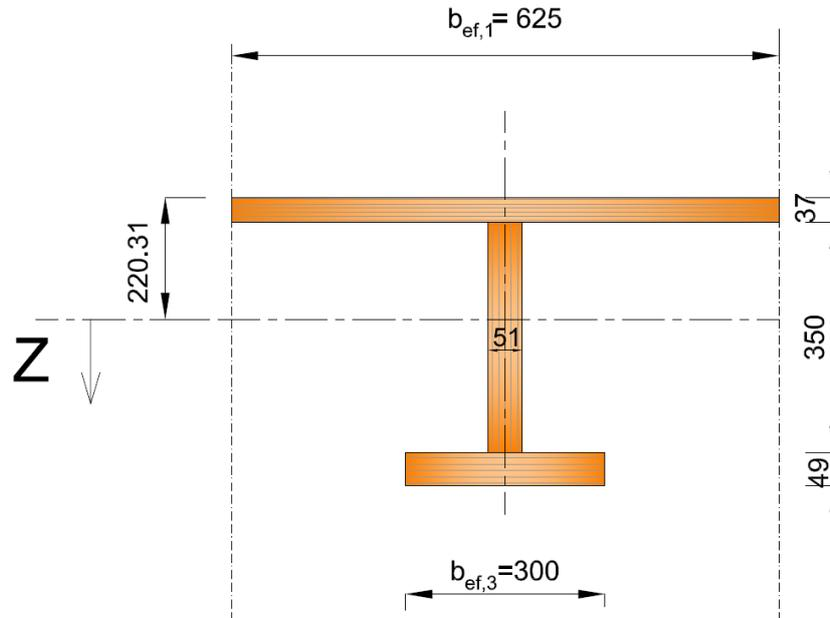
Figure 74: I section in SLS ( $t = \infty$ ) creep
