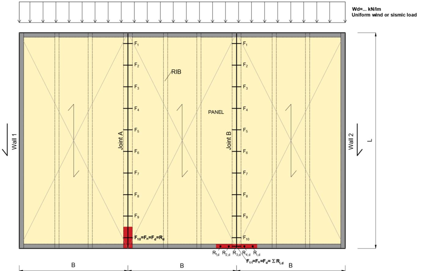
Figure 41: Fasteners placed in longitudinal joints and determination of the design carrying capacity of the outermost lying fastener  $F_d$  – Left (Joint A): Single fastener at the end; Right (Joint B): Multiple fasteners at the end.
