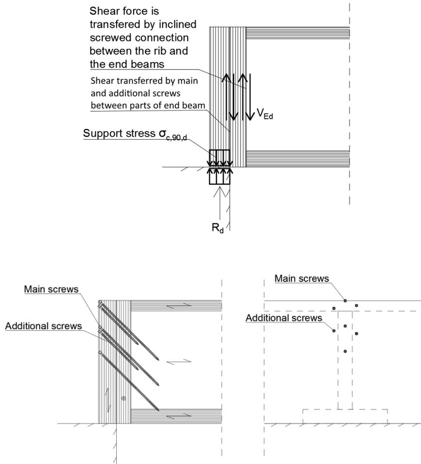
Figure 50: End beam support. Support reaction is transferred to shear force in ribs through end beam. ( $V_{ed} = R_d$ )
