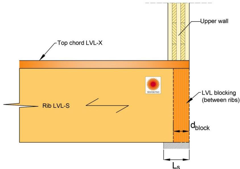
Figure 46: LVL Rib Panel simple support with wall above – Open.
