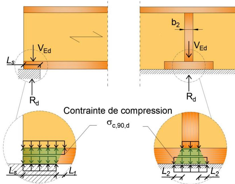
Figure 42: Effective contact area and stress distribution at a support.
