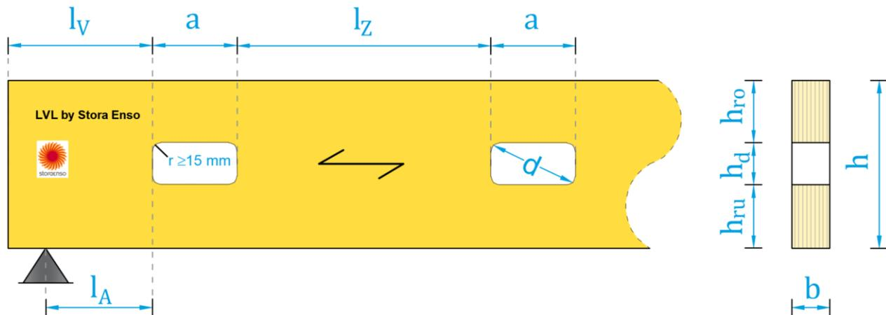
Figure 12: Definitions of geometric dimensions related to rectangular holes.
