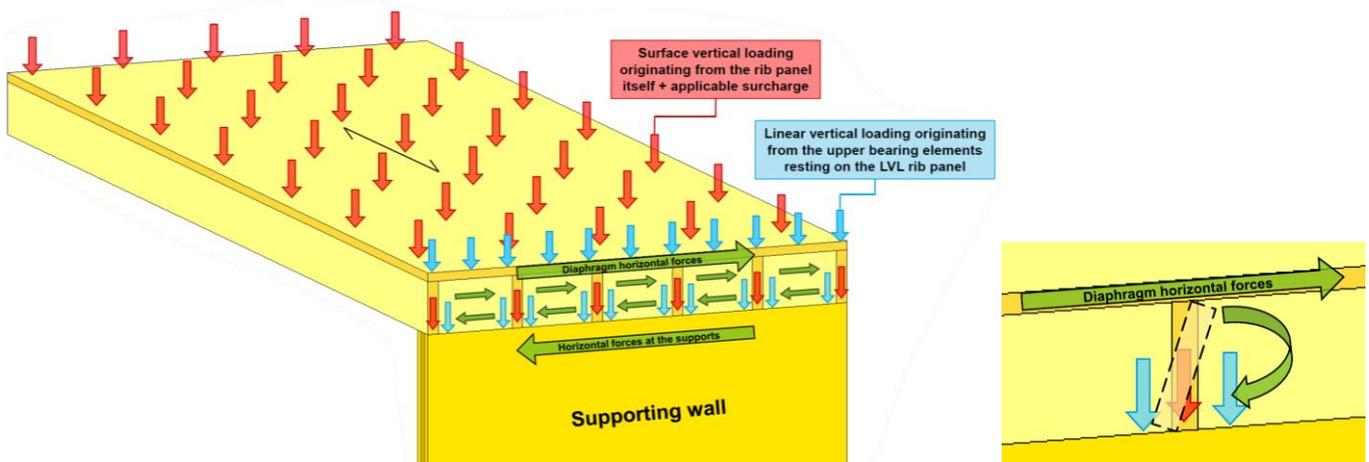
Figure 7: Load distribution into simple supports through blockings (blue) and through ribs (red)
