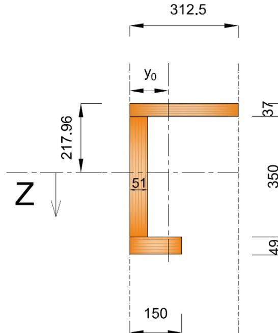
Figure 77: U section in SLS ( $t = \infty$ ) creep
