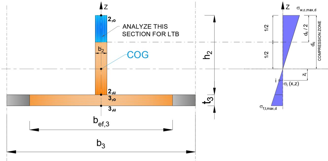
Figure 29: Inverted section for lateral torsional buckling analysis
