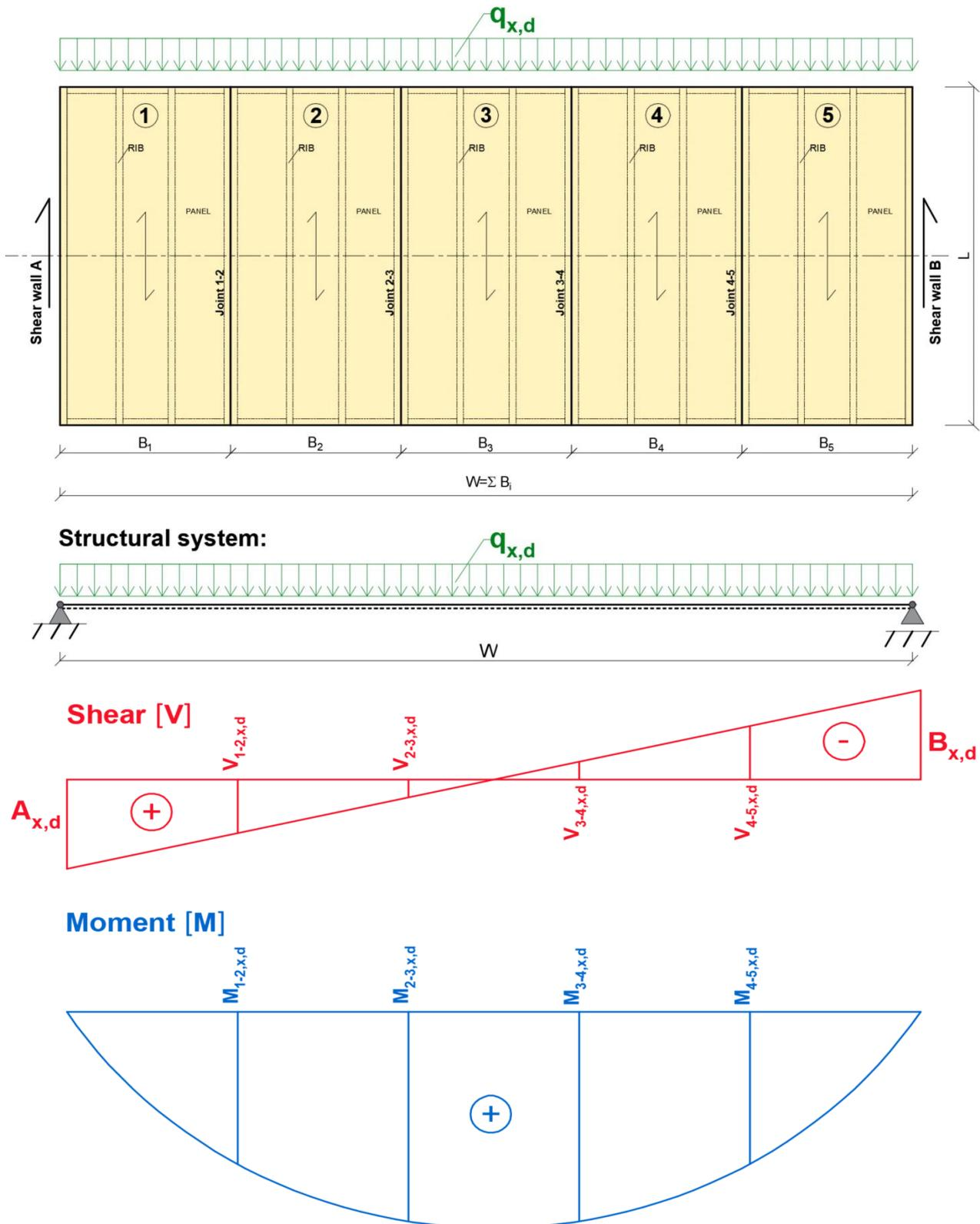
Figure 38: Modelling of LVL rib panels diaphragm in the direction of the span
