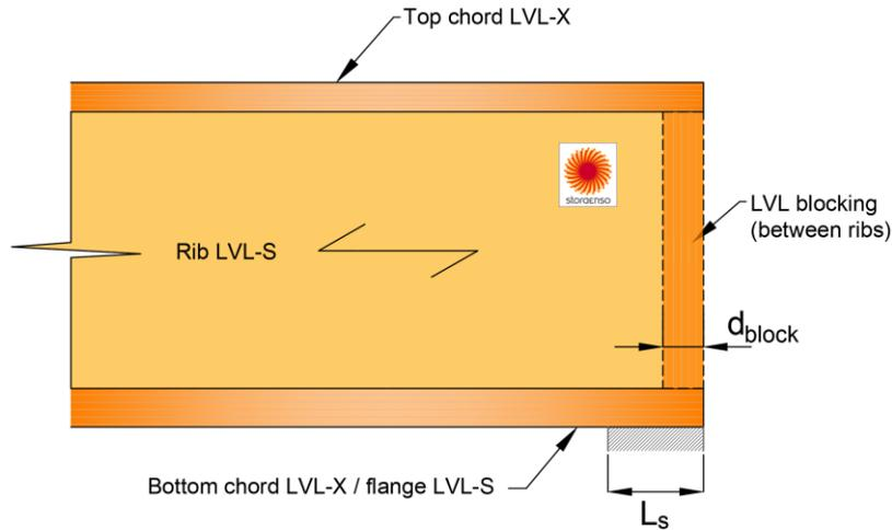
Figure 45: LVL Rib Panel simple support – Semi-Open/Closed/Inverted.
