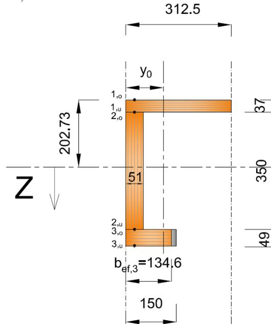
Figure 70: The calculation points of bending stress ( $t = \infty$ )
