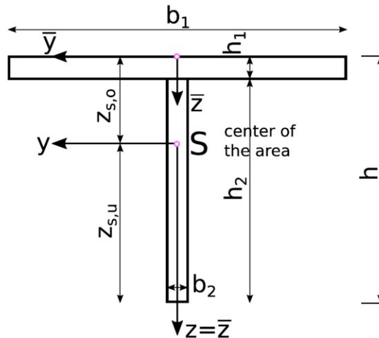
Figure 23: Geometry and notation of the T-shaped cross section
