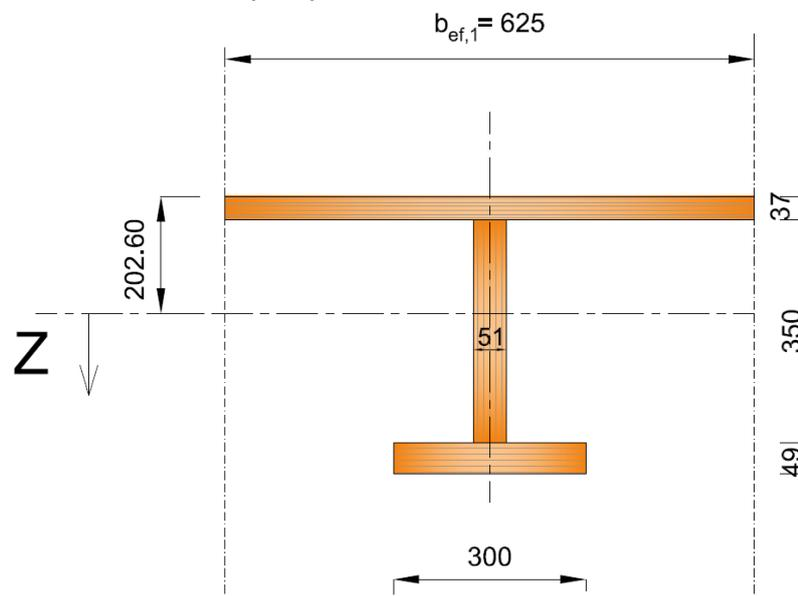
Figure 73: I section in SLS ( $t=0$ )
