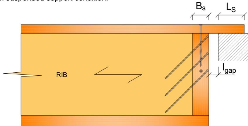
Figure 56: Suspension support geometry parameters.
