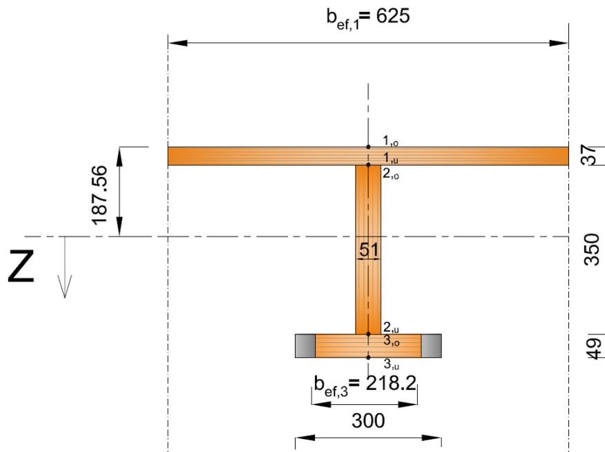
Figure 64: The calculation points of bending stress ( $t = \infty$ )
