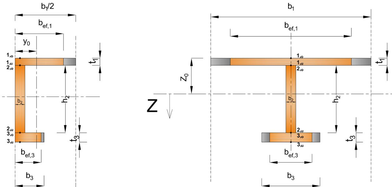
Figure 25: Calculation points of bending stress for rib panel.
