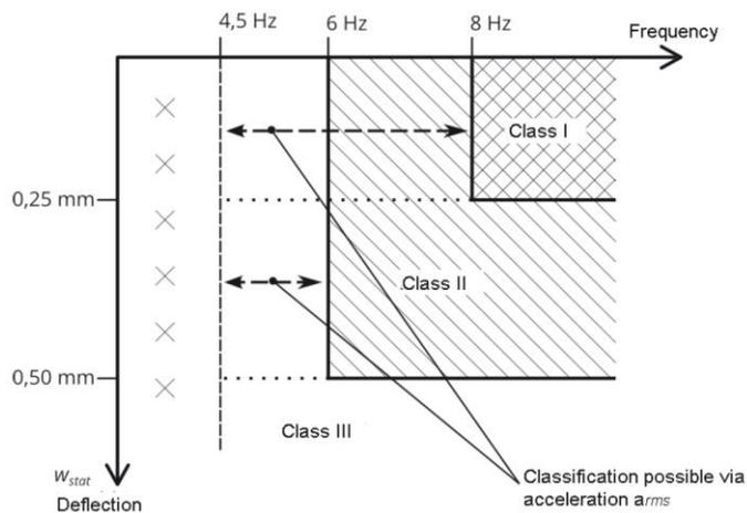
Figure 17: Vibration design flow chart
