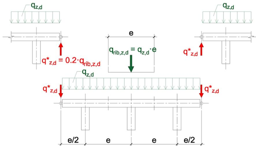
Figure 35: Design load  $q^*_{z,d}$  for longitudinal joints.
