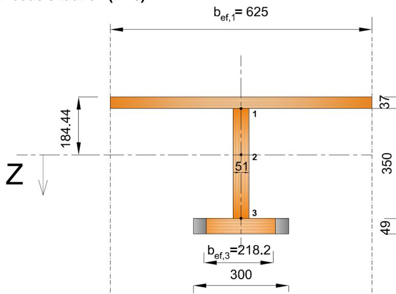
Figure 65: The calculation points of shear stress ( $t = 0$ )
