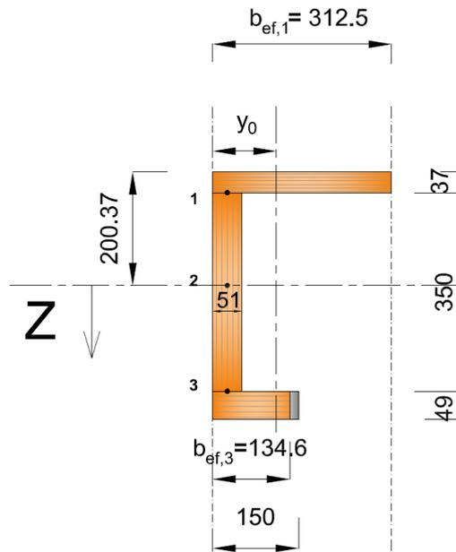
Figure 71: The calculation points of shear stress. ( $t = 0$ )
