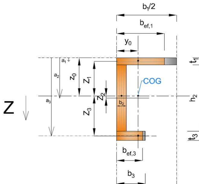
Figure 22; Cross section area- U section
