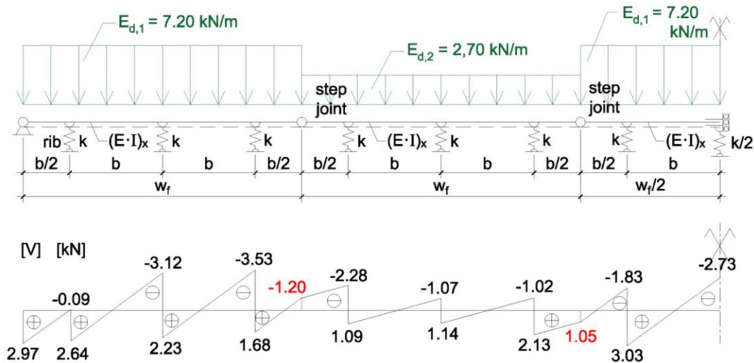
Figure 36: Analysed model and distribution of vertical forces
