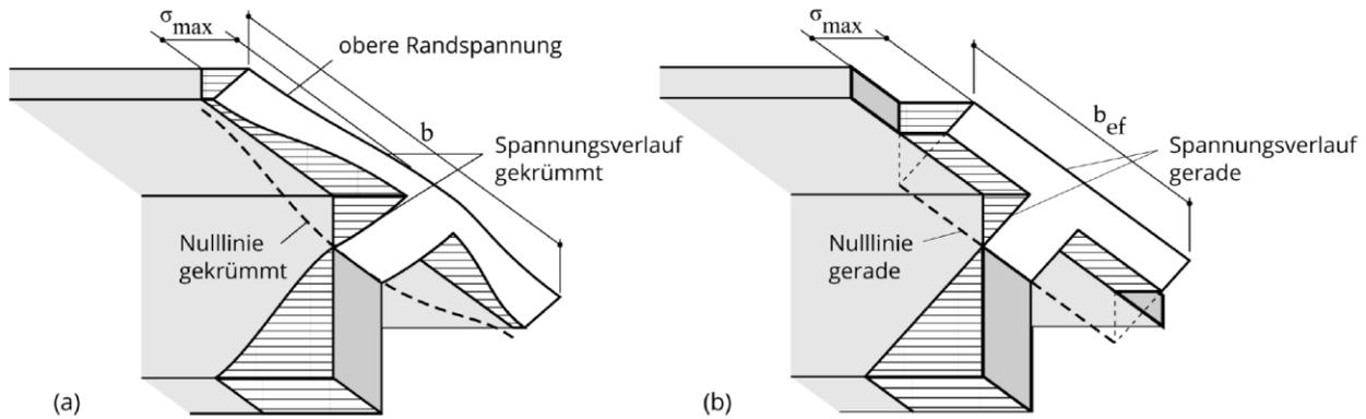
Figure 20: Effective width with (a) the actual stress distribution and (b) the linear stress distribution and effective width
