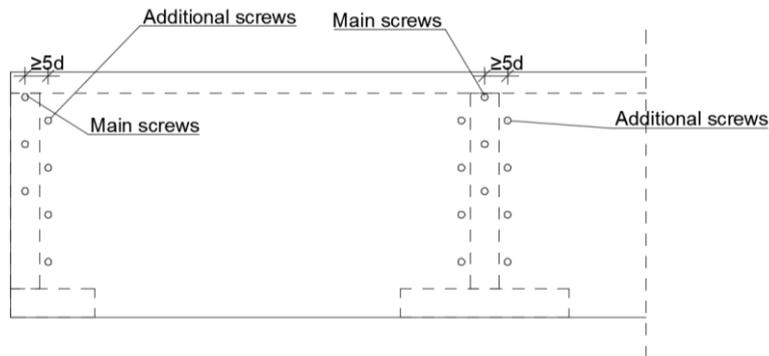
Figure 53: Screw instruction for additional screws.
