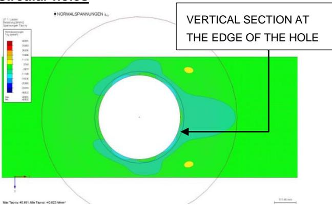
Figure 15: Shear stress distribution at the contour of a circular hole
