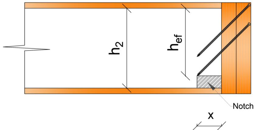
Figure 54: Determination of distances  $x$  and  $h_{ef}$ .
