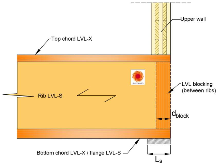
Figure 47: LVL Rib Panel simple support with wall above – Semi-Open/Closed/Inverted.
