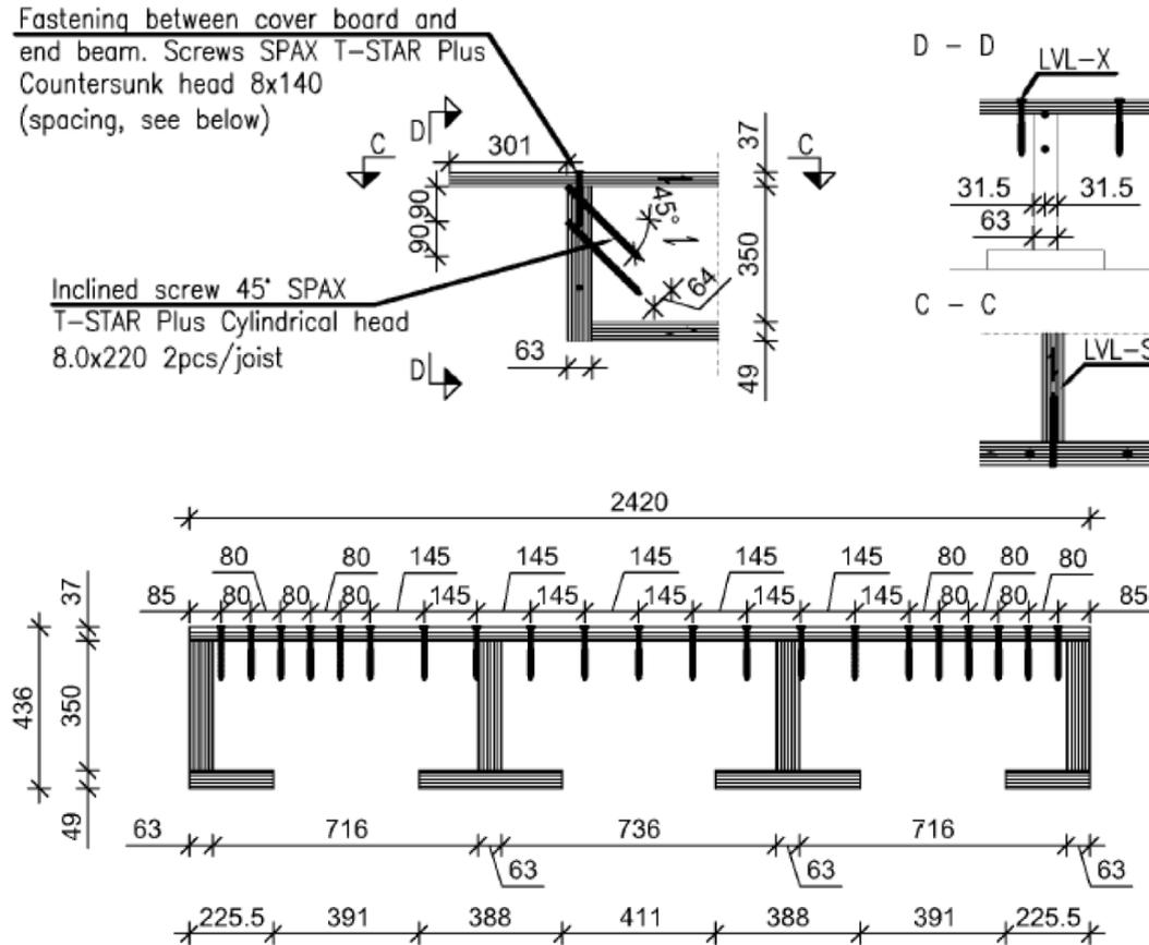
Figure 79: I section beam support and cross-section showing the position of suspension screws.
