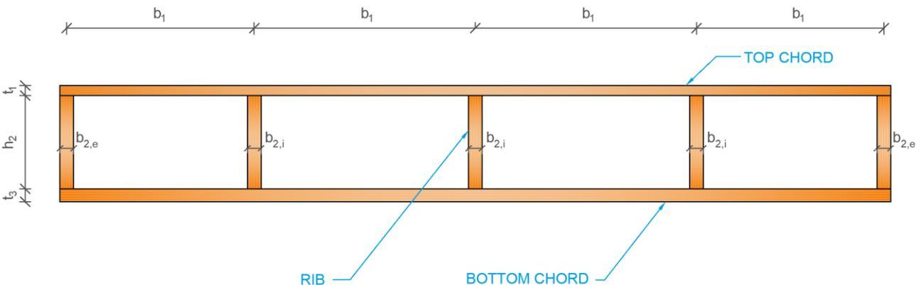
Figure 4: LVL Rib panel- Closed type.
