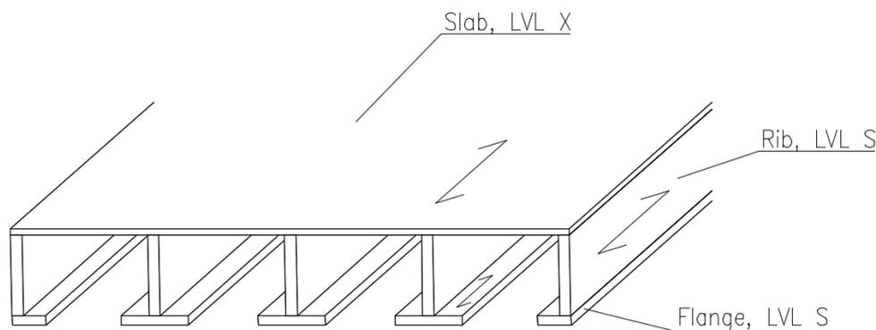
Figure 1: Rib panel. Arrows shows the main direction of grains.
