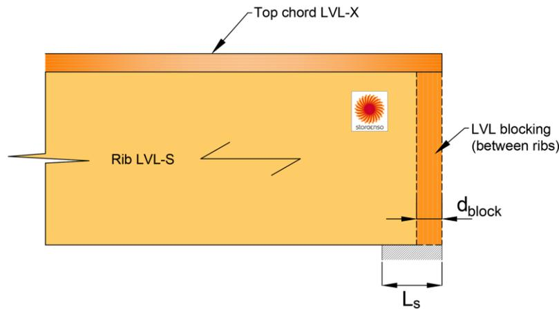
Figure 44: LVL Rib Panel simple support - Open
