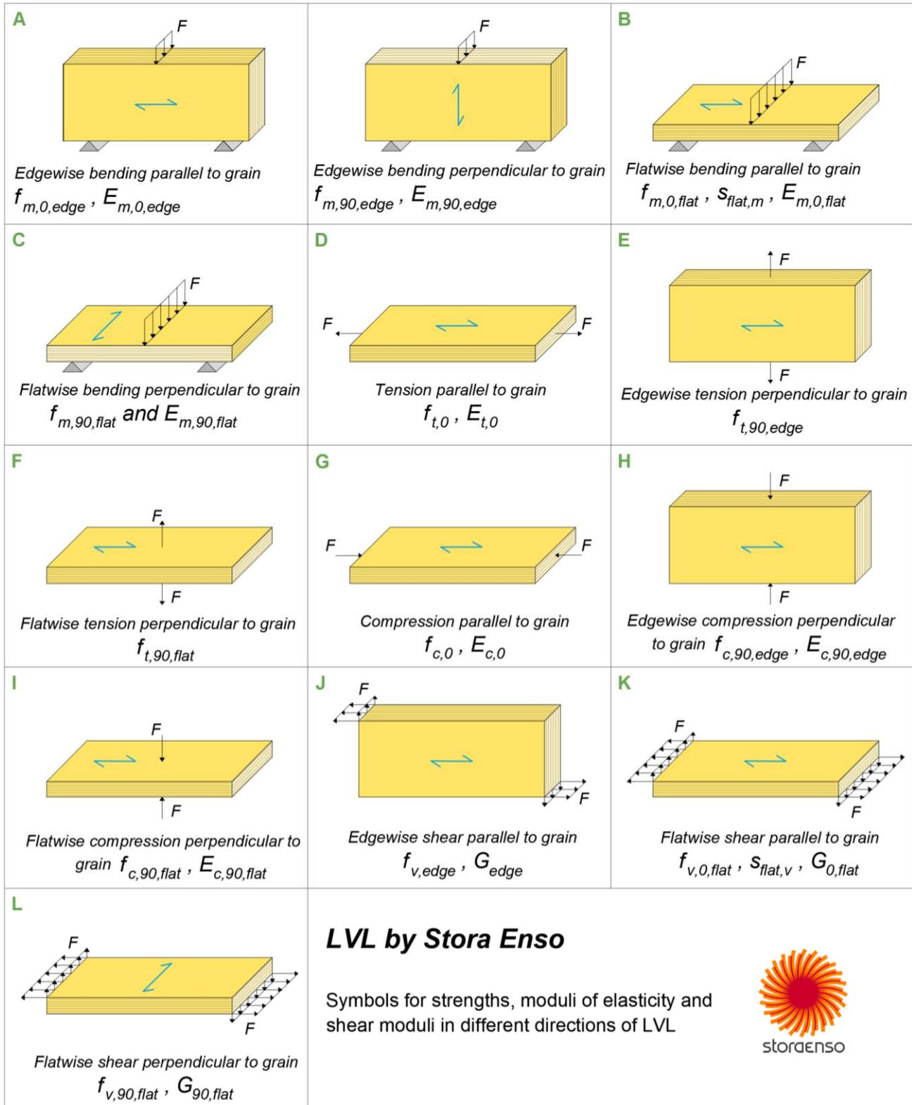
Figure 10: Strength and stiffness orientations.
