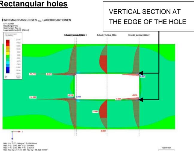
Figure 14: Shear stress distribution at the contour of a rectangular hole
