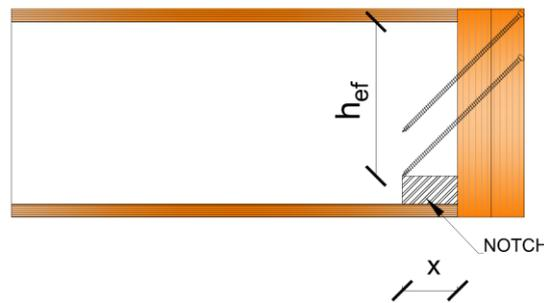
Figure 80: Determination of distances  $x$  and  $h_{ef}$  (should be adapted to the suspended support example)
