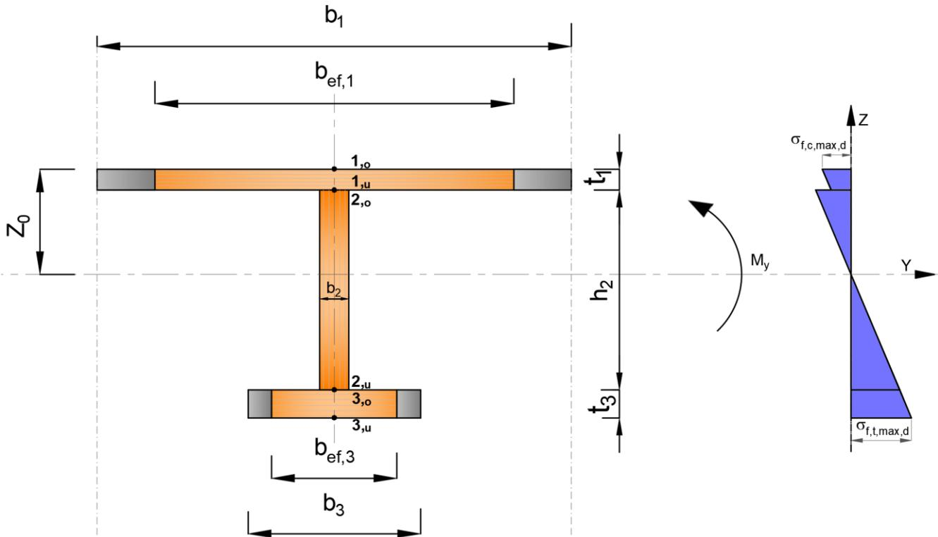
Figure 26: Bending stress distribution
