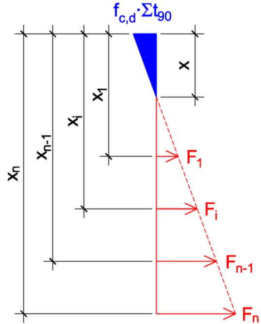
Figure 39: Compression zone perpendicular to grain (blue) at the edge of the joint and tension zone (red) with the load carrying capacity of the outermost lying fastener.
