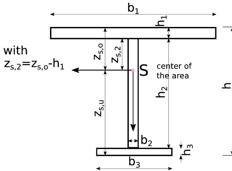
Figure 24: Geometry and notation of the I-shaped cross section
