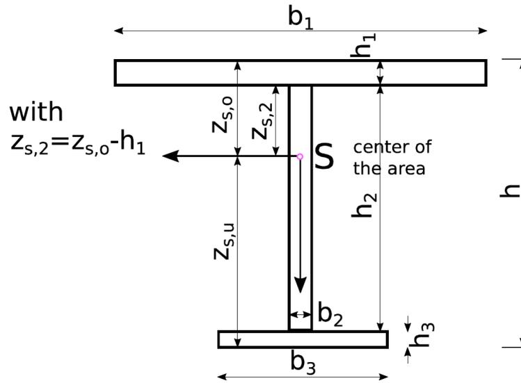
Figure 75:I shaped cross section
