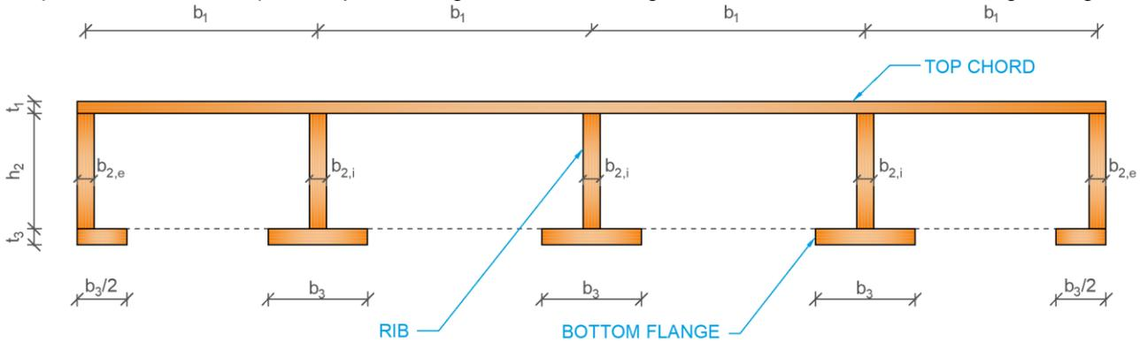
Figure 3: LVL Rib panel- Semi open type.
