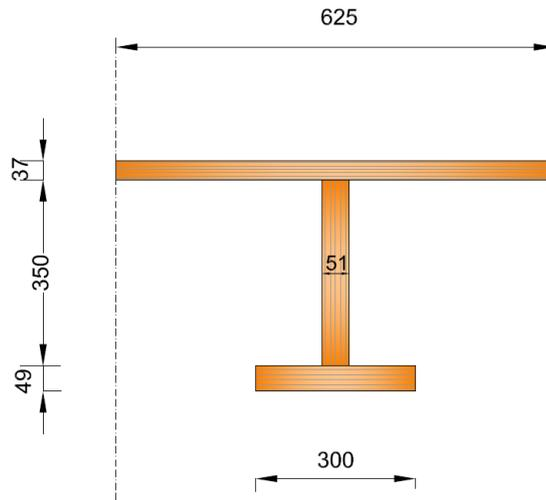
Figure 61: I section dimension
