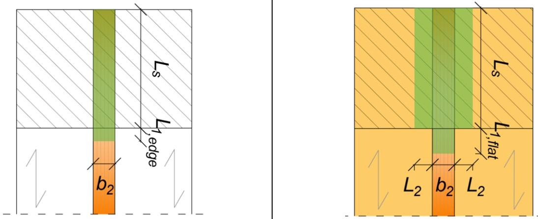
Figure 43: Load bearing area of the different part of the LVL Rib Panel section.
