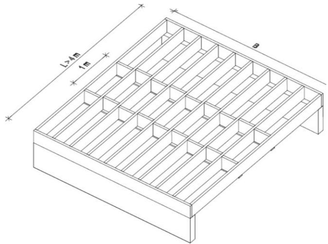
Figure 9: Two lines of blockings for span >4m
