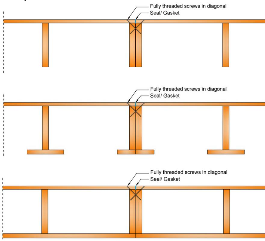
Figure 32: Assembly of adjacent LVL Rib Panels by means of diagonal screwed connection at the edge ribs.
