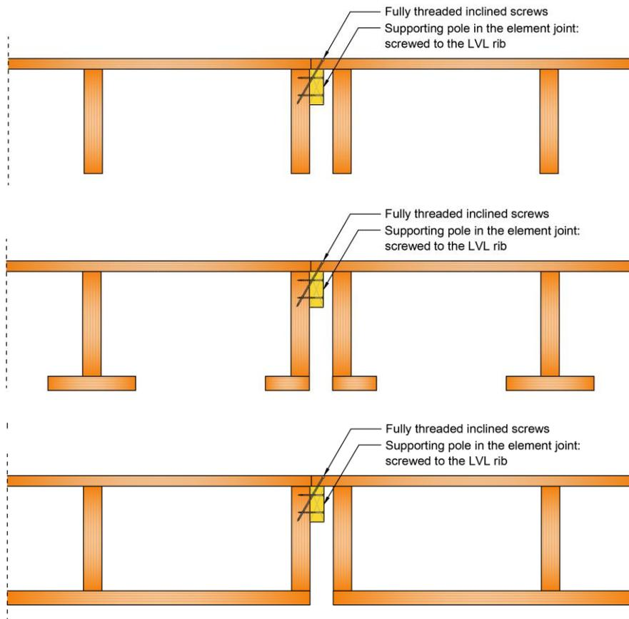
Figure 33: Assembly of adjacent LVL Rib Panels by means of supporting pole screwed at the edge ribs.
