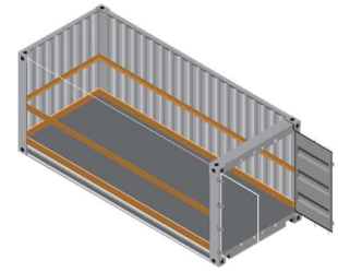
Side protection on container walls
