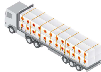
Securing of timber packages
