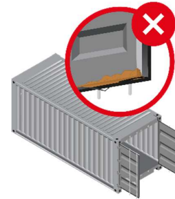
Rust on doors
