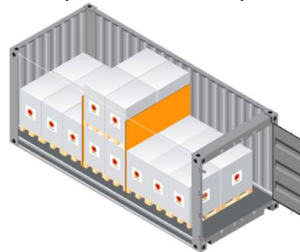
Threshold by pane. Board used to block pallets.
