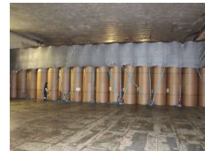
Cargo securing in StoRo vessel
