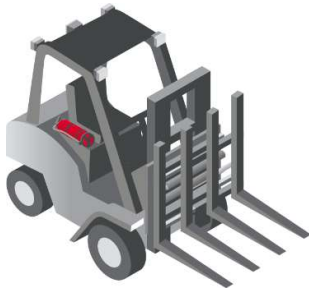
Forklift with double pallet handlers
