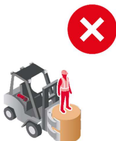
Do not stand on top of the load
