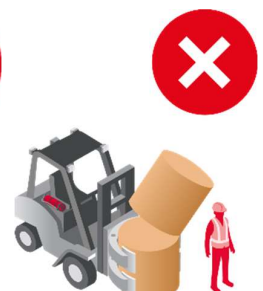
No loose (unclamped) reels/ No free riders
