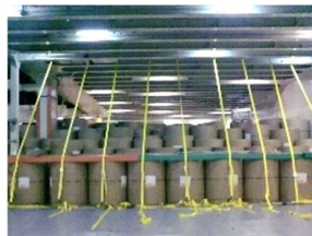
Cargo securing in StoRo vessel
